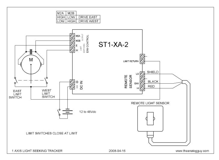
The ST1-10 and 20A are light seeking tracker controls designed for DC motor systems. In unobstructed sunlight it typically tracks within one degree of actual sun position.
