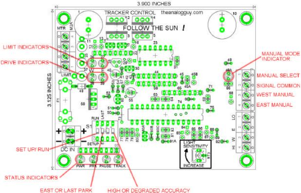
The pcb assembly needs to be mounted indoors or in a weatherproof enclosure.
