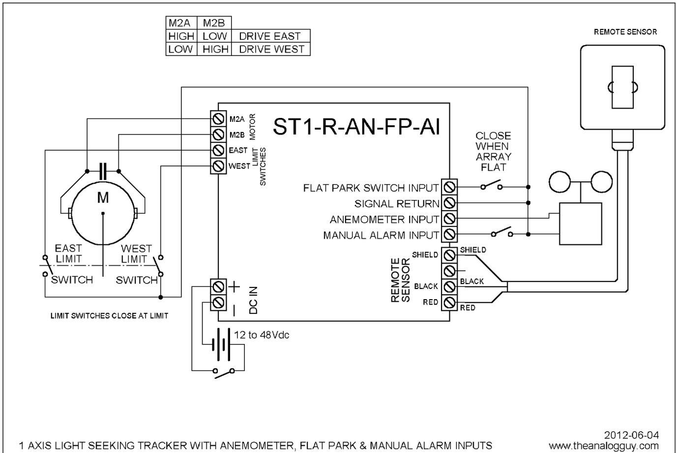
The ST1-10 and 20A are light seeking tracker controls designed for DC motor systems. In unobstructed sunlight it typically tracks within one degree of actual sun position.
