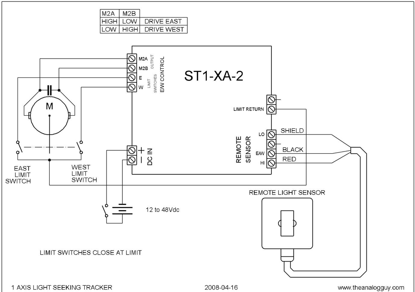
The ST1-5 and 10A is are light seeking tracker controls designed for DC motor systems. In unobstructed sunlight it typically tracks within one degree of actual sun position.
