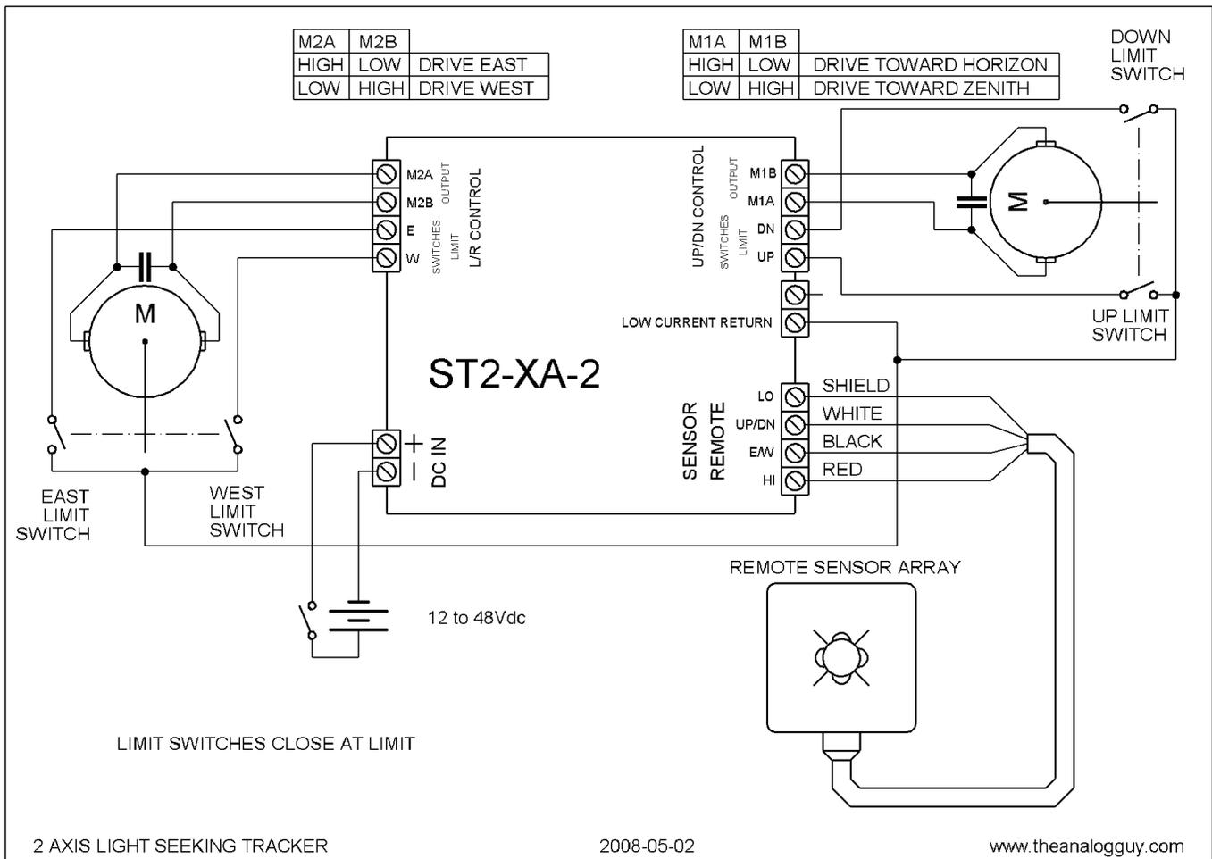
The ST2-10A is a light seeking tracker control designed for DC motor systems (typically linear actuators) with up to 48VDC maximum operating voltage (minimum operating voltage=10VDC, maximum allowable voltage=56vdc). In unobstructed sunlight it typically tracks within one degree of actual sun position. After the power up, the ambient light level will determine the operating mode.
