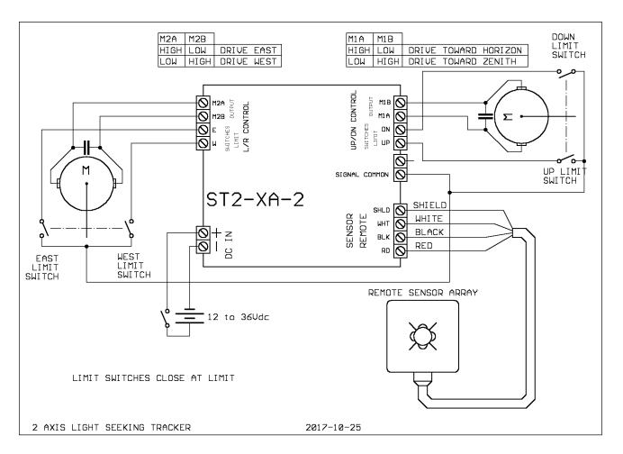
The ST2-10A and ST2-20A are light seeking tracker controls designed for DC motor systems (typically linear actuators) with up to 36VDC maximum operating voltage (minimum operating voltage=10VDC, maximum allowable voltage=36vdc). In unobstructed sunlight it typically tracks within one degree of actual sun position.
