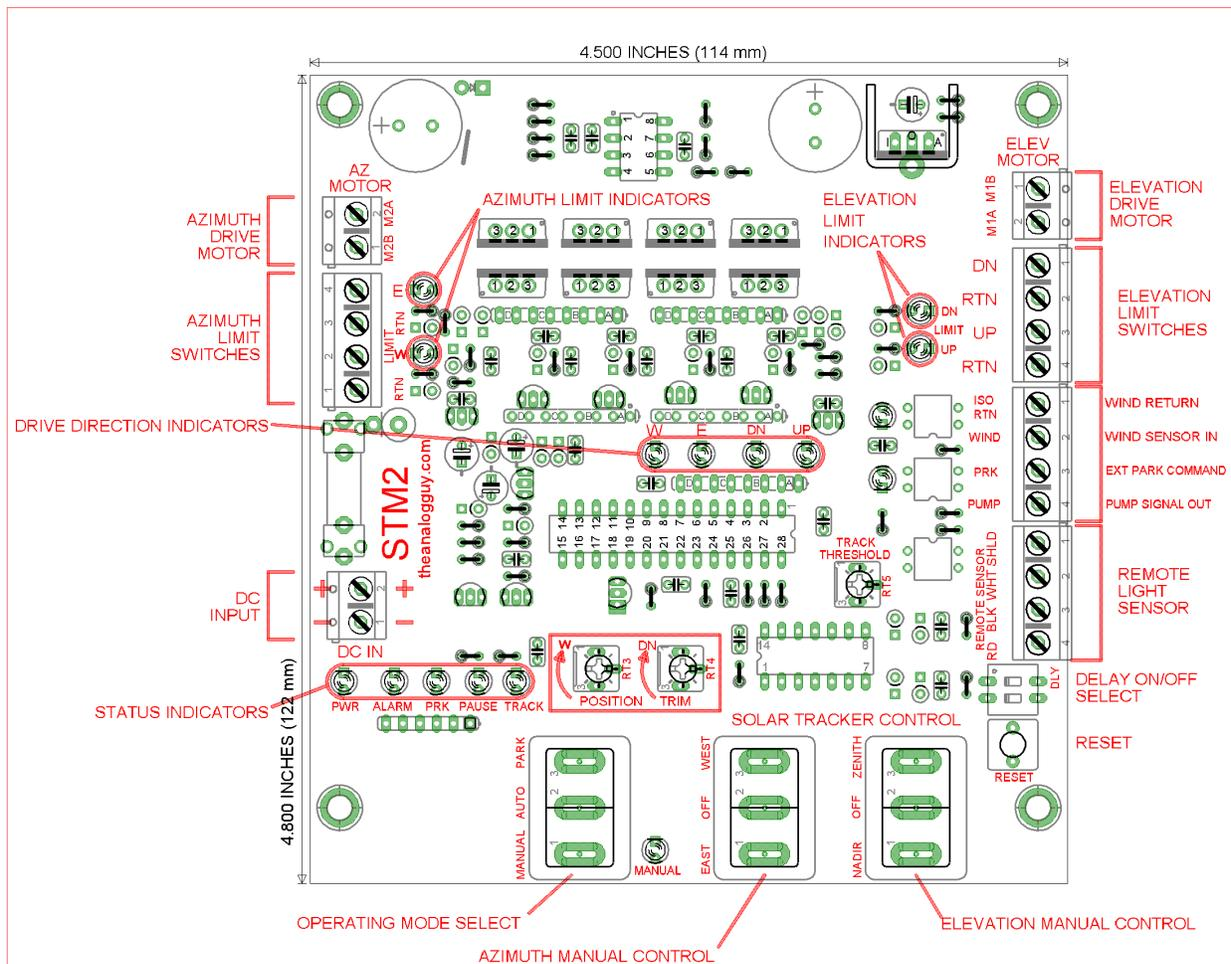
The STM2-20A is a light seeking tracker control designed for DC motor systems. It has a manual control capability and wind alarm input.
