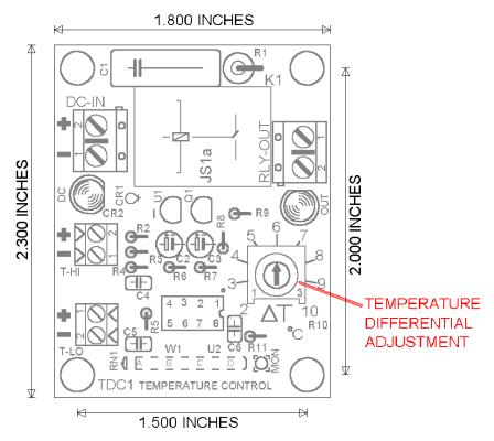
The TDC1 is a temperature differential temperature control that provides a normally open relay contact that closes when T-HI = T-LO + delta T. Delta T is adjustable from 2 to 10 degrees C.
